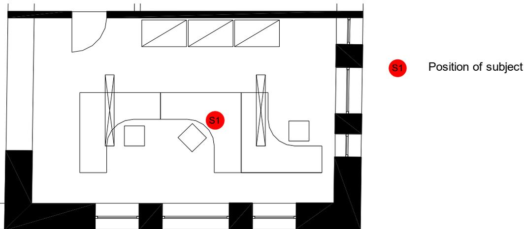
Figure 4.13: Detailed view of the single-occupant office with an indication of the subject's position.
