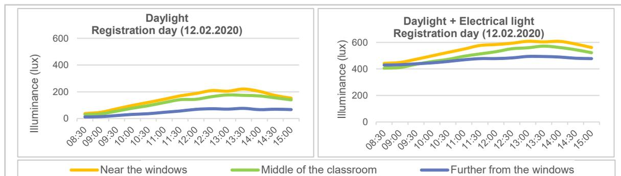
Figure 4.49 Registration Day, illuminance on task position Daylight (left) and Daylight + Electrical light
