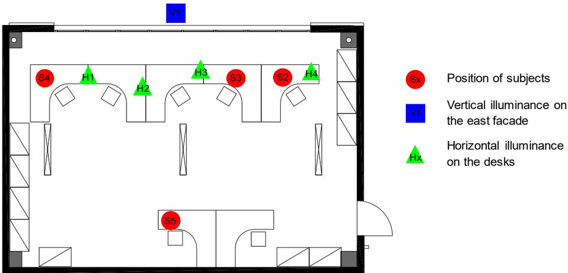
Figure 4.12: Detailed view of the multi-occupant office with an indication about the indoor illuminance values measurement points as well as the position of the employees.
