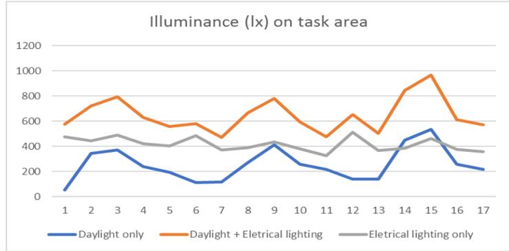
Figure 4.41 Diagram of task light level on each task area in 3 scenarios.
