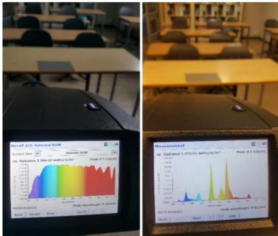
**Figure 4.27: Registration of spectrum power distribution of lighting in space; daylight (left) and fluorescent lamp (right); by spectroradiometer.**
