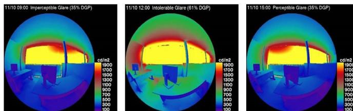
Figure 9. Point in time glare in South facing room, 10<sup>th</sup> November at 9 a.m. (left), 12 p.m. (center) and 3 p.m. (right) with clear sky.
